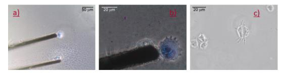
Cell membrane permeabilization verification with trypan blue (TB) staining after electroporation: a) electrodes next to the target cells before electroporation, b) cell in vicinity of the electrode after electroporation – TB localized I the cell, c) unaffected cells not stained with TB [1].
