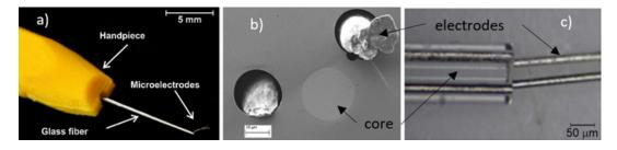
Thin glass fiber microprobe for electroporation of selected cells: a) entire device; zoomed electrodes and high refractive index core b) front view and c) side view [1].
